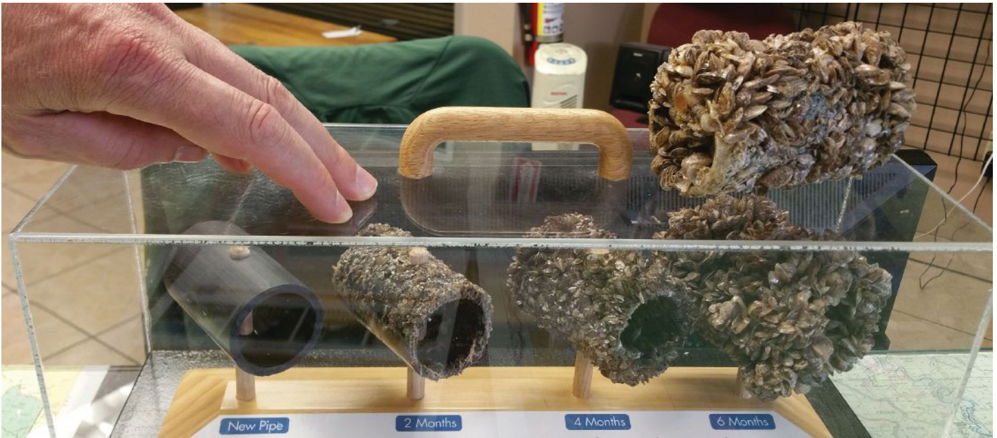
Quagga mussels at different stages on a pipe.
